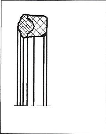
The compact rod seal is an inseparable sealing element, which is consisting of a cotton fabric reinforced rubber U-ring and a rubber part. The rubber part of the compact rod seal ensures excellent sealing performance at high and low pressures. The fabrics reinforced rubber U-ring forms an oil layer at the sealing surface, which reduces friction and extrusion of the compact rod seal and extends the operating life time.
