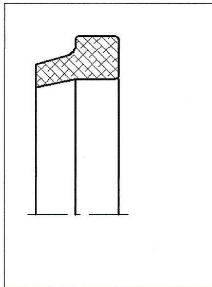
The function of wiper is to remove mechanical and other impurities from the piston rod and thus prevent damage to the guide ring and the seal. The lip of the wiper removes even the finest dirt from the piston rod, and prevents it from penetrating into the cylinder tube, and thus extrusion of moving parts of the assembly.
