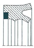
This seal is mostly used for sealing telescopic cylinders.
