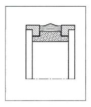
Sealing setR-83 is used for sealing pistons for hydraulic cylinder. Sealing set R-83consists of anreinforced ring elastomer-fabric manufactured from NBR ,elastomeric spring manufactured from NBR and two guiding rings manufactured from polyacetal.
