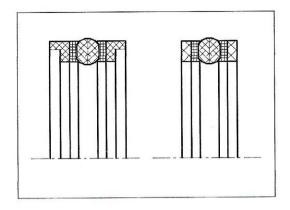
Sealing set SIMKO 5 is to be installed onto pistons of hydraulic cylinders.
